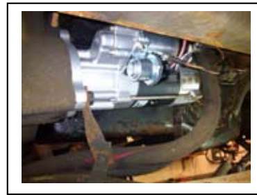
M105R2517SE mounted on bus engine
